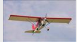
The spinner is the aerodynamic nose cone that fits on the front of the propeller. Source: MIT
